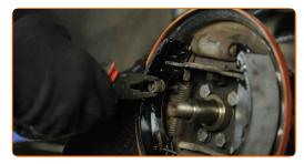
27 Install the brake pads retaining clips. Use pliers.
