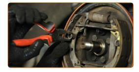
Pull both brake shoes with the adjuster from the working brake cylinder, avoiding damage to the boots.
