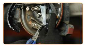
Attach the brake shoes, together with the brake adjuster, to the wheel cylinder.
