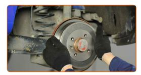
Tigten the brake drum fasteners. Use a Phillips screwdriver. Use a torque wrench. Tighten it to 4 Nm torque.
