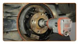
Install the hub bearing protection cap. Use a rubber mallet.
