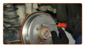
Remove the brake drum.
