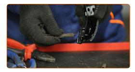
Place the brake shoes so that their inward edges rest on the anchor plate.
