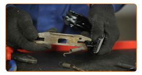
Install the retaining springs of the brake pads. Use round-nose pliers.
