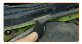
Unscrew the plastic panel fasteners. Use a Phillips screwdriver.
