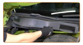
Screw on the plastic panel fasteners. Use a Phillips screwdriver.
