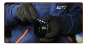
Install a new O-ring to its mounting seat on the filter cover. Use a flat screwdriver.
