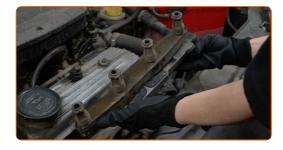
Clean dirt, dust and debris from inside the spark plug wells.
