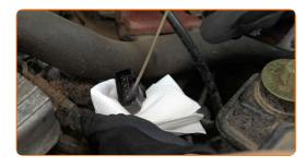
Plug in the ignition coil connector.
