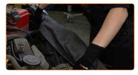
Detach the connector from the ignition coil.
