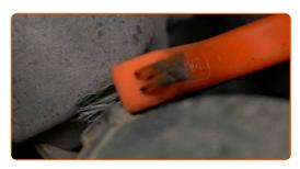
Unscrew the ignition coil bolts. Use a drive socket #10. Use a ratchet wrench.
