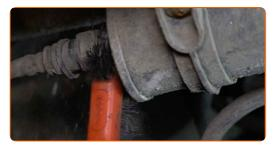
Squeeze the clips and detach the fuel supply lines from the fuel filter housing.
