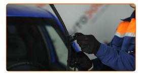
Remove the blade from the wiper arm.
