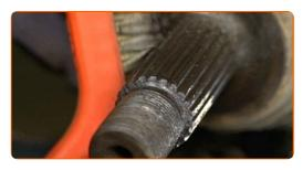
Treat the splines of the driveshaft CV joint. Use copper grease.
