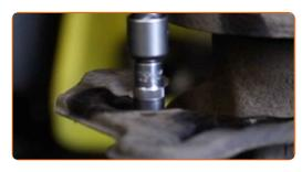
Remove the brake disc cover.
