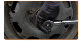
Tighten the wheel bolts using a criss-cross pattern. Use wheel impact socket #17. Use a torque wrench. Tighten it to 110 Nm torque.
