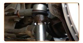
Tighten the fasteners connecting the ball joint to the control arm. Use a drive socket #13. Use a torque wrench. Tighten it to 20 Nm torque. +90°
