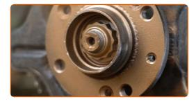
69 Install the brake disc.
