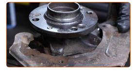
Tighten the fasteners of the brake disc back plate. Use a drive socket #8. Use a torque wrench. Tighten it to 5 Nm torque.
