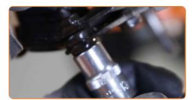
Detach the driveshaft from the steering knuckle. Use a pin punch. Use a hammer.
