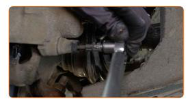
Treat the fasteners of the ball joint. Treat the shock strut fasteners. Treat the fastener connecting the tie rod end to the steering knuckle. Use copper grease.
