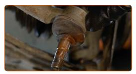
Connect the tie rod end to the steering knuckle.
