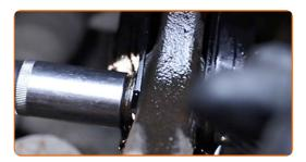
Clean the fasteners connecting the ball joint to the suspension control arm. Use a wire brush. Use WD-40 spray.
