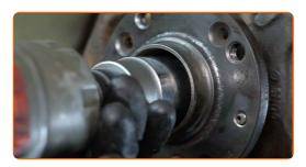
Clean the mounting seat of the tie rod end. Use a wire brush. Use WD-40 spray.
