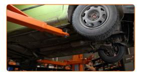
Tighten the drive shaft nut. Use a drive socket #30. Use a torque wrench. Tighten it to 175 Nm torque.
