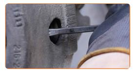
10 Remove the brake caliper.
