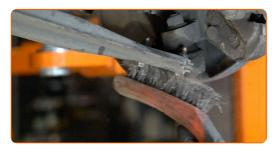
Unscrew the ball joint fastening to the steering knuckle. Use a combination spanner #17. Use a ratchet wrench.
