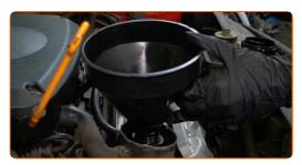
Pour oil into the engine through the filler. Required amount of oil: 4.4 l.
