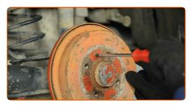
Remove the brake drum.
