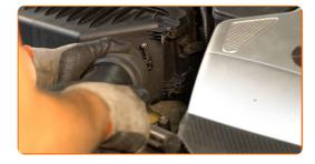
Secure the fastener of the air intake duct. Use a drive socket #10. Use a ratchet wrench.
