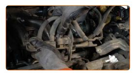
79 Screw in the vacuum system bracket. Use a drive socket #12. Use a ratchet wrench.
