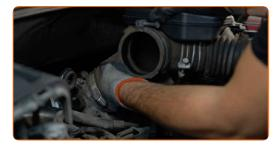
Screw in the clamp that connects the air filter hose to the throttle body. Use a drive socket #10. Use a ratchet wrench.
