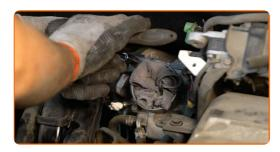
Detach the throttle body from the intake manifold.
