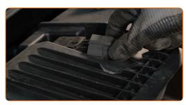
Unscrew the air intake resonator clamp from the air filter housing. Use a drive socket #10. Use a ratchet wrench.
