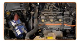
Unscrew the air filter housing bracket. Use a drive socket #12. Use a ratchet wrench.
