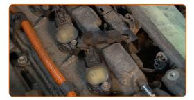
Clean the intake manifold mounting seats. Use all-purpose cleaning spray.
