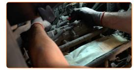
Unscrew the fasteners of the ignition coils. Use a drive socket #10. Use a ratchet wrench.
