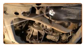
Screw in the new drainage plug and tighten it. Use a drive socket #14. Use a torque wrench. Tighten it to 27 Nm torque.
