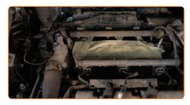
Cover the intake channels of the engine with a microfibre cloth to prevent dust and dirt from getting inside.
