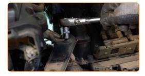
Detach the crankcase ventilation hose clamp. Use clic-R collar pliers.
