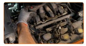
Clean the intake manifold fasteners.
