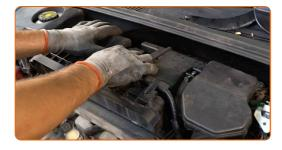
Install the battery cover. Reinstall the battery cover clips.
