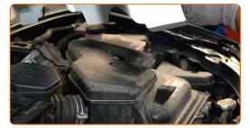
Unscrew the air filter box fasteners. Use a drive socket #10. Use a ratchet wrench.
