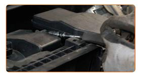
Unscrew the filter housing fastening bolts. Use a drive socket #10. Use a ratchet wrench.
