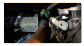
Tighten the intake manifold fasteners. Use a drive socket #14. Use a torque wrench. Tighten it to 15 nm torque.
