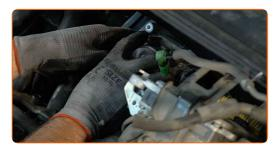
73 Tighten the throttle valve fasteners. Use a drive socket #12. Use a ratchet wrench.
