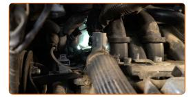
Detach the crankcase ventilation hose clamp.
