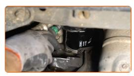
Clean the area of the oil pan drainage hole. Use all-purpose cleaning spray.
