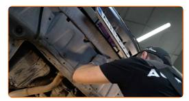
Tighten the fasteners of the oil pan lower cover. Use a drive socket #10. Use a ratchet wrench.
