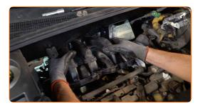
Tighten the intake manifold fasteners. Use HEX No.H8. Use a ratchet wrench.
