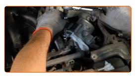
Tighten the intake manifold fasteners. Use a drive socket #12. Use a ratchet wrench.
