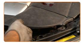
Remove the engine cover clips.
