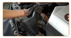
Release the air filter cover clips.
