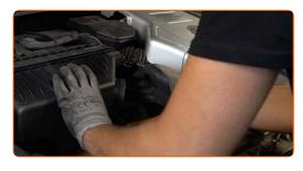
100 Install the air duct housing.
