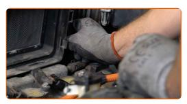
Screw in the air intake resonator clamp to the air filter housing. Use a drive socket #10. Use a ratchet wrench.
