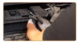
19 Remove the air filter housing.
