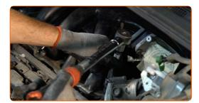
Tighten the intake manifold fasteners. Use HEX No.H8. Use a torque wrench. Tighten it to 15 nm torque.
