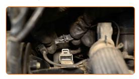
Attach the throttle valve connectors.
