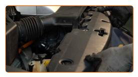
104 Install the radiator support cover clips.
