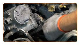
78 Attach the vacuum sensor connector.
