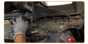
Screw the fastening clamp connecting the air duct to the air filter housing. Use a drive socket #10. Use a ratchet wrench.
