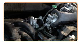
Clean the throttle body fasteners. Use all-purpose cleaning spray.
