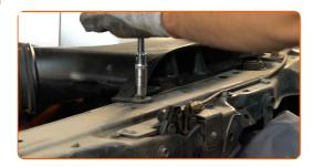
Loosen the fastening clamp connecting the air duct to the air filter housing. Use a drive socket #10. Use a ratchet wrench.
