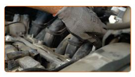
Detach the throttle valve connectors.
