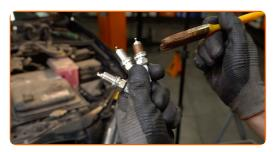
Install the new spark plugs into their mounting seats. Use the spark plug socket #16. Use a ratchet wrench.
