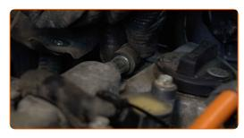
Install the clamp of the crankcase ventilation hose. Use clic-R collar pliers.
