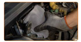
Unscrew the vacuum system bracket. Use a drive socket #12. Use a ratchet wrench.
