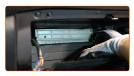
Remove the cabin air filter housing.
