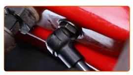
13 Install the new boot lid gas strut.
