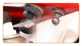
10 Install the new boot lid gas strut.
