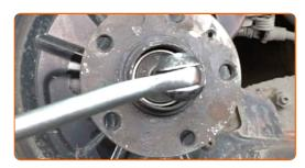
Remove the fastening bolt.
