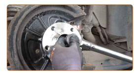
28 Install the hub bearing protection cap. Use a rubber mallet.
