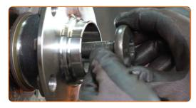
Tighten the hub. Use XZN #18. Use a torque wrench. Tighten it to 180 nm torque.
