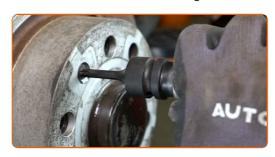
18 Remove the brake disc.
