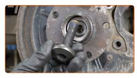
Remove the hub and the bearing together, since they are a sealed unit.
