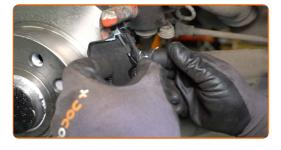
Install the brake caliper and fix it.
