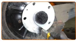
31 Install the brake disc.
