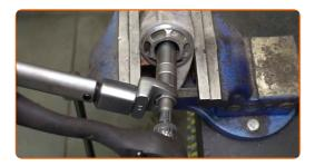
Treat the shock absorber rod fastener. Use copper grease.
