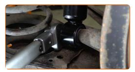
Tighten the shock absorber mount fasteners. Use a drive socket #16. Use a torque wrench. Tighten it to 50 Nm torque.+45°
