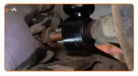
Screw in the lower fastener of the shock absorber. Use a combination spanner #21.
