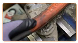
Remove the shock absorber piston rod fastening. Use a drive socket #16. Use a shock absorber socket DDNº5,2. Use a ratchet wrench.
