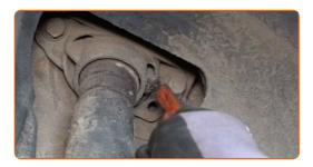
Unscrew the shock absorber mount fasteners. Use a drive socket #16. Use a ratchet wrench.
