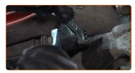
Remove the brake caliper. Use a crowbar.
