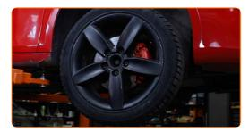
Tighten the bolt connecting the drive shaft to the wheel hub. Use 12-point socket No.24. Use a torque wrench. Tighten it to 70 Nm torque.+90°
