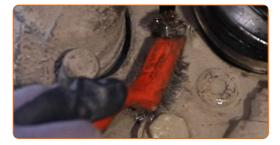
Unscrew the brake caliper bracket fasteners. Use a drive socket #21. Use a ratchet wrench.
