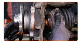
Install and tighten the drive shaft bolt. Use 12-point socket No.24. Use a ratchet wrench.
