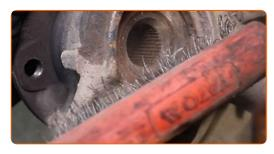
Unscrew the wheel hub bolts. Use XZN #12. Use a tap wrench.
