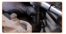
Tighten the fastener connecting the stabilizer link to the shock strut. Use a drive socket #18. Use XZN #6. Use a torque wrench. Tighten it to 65 Nm torque.
