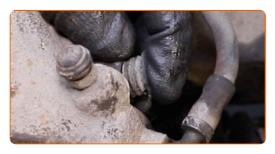
Install the brake caliper retaining spring.
