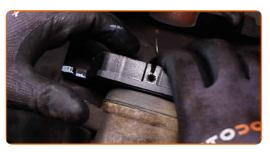
Install the brake caliper and fix it. Use HEX No.H7. Use a ratchet wrench.
