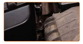
Remove the fender protection cover.
