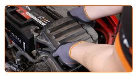
Unscrew the filter element fastener. Use a Phillips screwdriver.
