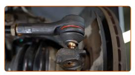
Set the tie rod end to the correct position and secure it with the lock nut. Use a vernier caliper. Use a combination spanner #19. Use a combination spanner #22.
