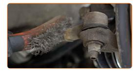
Loosen the lock nut securing the tie rod end to the tie rod. Use a combination spanner #19. Use a combination spanner #22.
