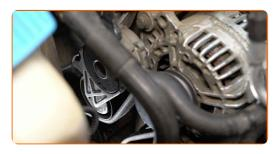
Rotate the crankshaft several times to check whether the new V-ribbed belt is working correctly. Use a drive socket #19. Use a ratchet wrench.
