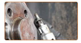
Remove the brake disc.
