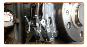
Install the brake caliper.
