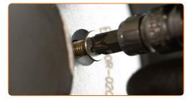
Tighten the brake disc fasteners. Use a Phillips screwdriver. Use a torque wrench. Tighten it to 4 Nm torque.
