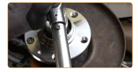
Install the hub bearing cap. Use a rubber mallet.
