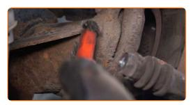
Unscrew the brake caliper bracket fasteners. Use HEX No.H8. Use a ratchet wrench.
