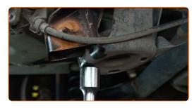
Unscrew the wheel hub fastener. Use 12-point socket No.30. Use a tap wrench.
