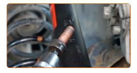
Remove the brake caliper bracket.
