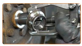
Clean the hub bearing mounting seat. Use a wire brush. Use all-purpose cleaning spray.
