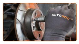
19 Remove the fastening bolt.
