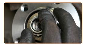
Tighten the hub fastener. Use 12-point socket No.30. Use a torque wrench. Tighten it to 175 Nm torque.
