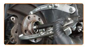
Remove the inner bearing ring from the stub axle. Use 3-Arm Gear Puller.
