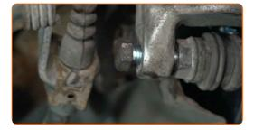
Tighten the brake caliper fasteners. Use a drive socket #13. Use a torque wrench. Tighten it to 35 Nm torque.
