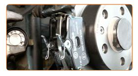
18 Install the brake caliper.
