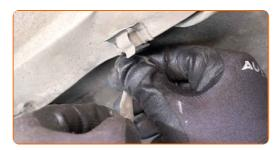
6 Clean the oxygen sensor fastener. Use a wire brush. Use WD-40 spray.
