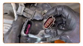
Disconnect the oxygen sensor wiring.
