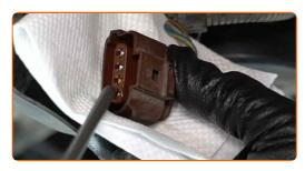
Attach the oxygen sensor connector.
