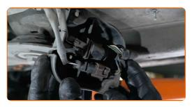
Detach the oxygen sensor connector.
