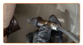
Clean the thread to prepare it for installing a new oxygen sensor. Use a thread tap. Use a ratchet wrench.
