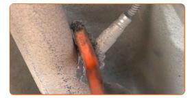
Unscrew the oxygen sensor fastener. Use a 22-mm oxygen sensor socket. Use a ratchet wrench.
