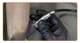
Tighten the oxygen sensor fastener. Use a 22-mm oxygen sensor socket. Use a torque wrench. Tighten it to 46 Nm torque.
