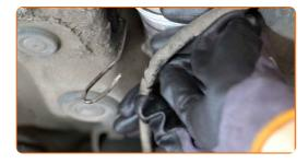
Loosen the fuel filter fasteners. Use a drive socket #7. Use a ratchet wrench.
