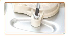
Unscrew the speaker's fasteners. Use a drive socket #8. Use a ratchet wrench.
