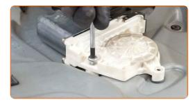
Remove the power window motor.
