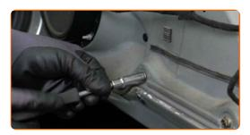
Unscrew the door lock fasteners. Use XZN #8. Use a ratchet wrench.
