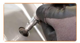
Tighten the door panel fasteners. Use a drive socket #10. Use a torque wrench. Tighten it to 8 Nm torque.
