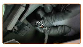
Unscrew the window glass fasteners. Use a drive socket #10. Use a ratchet wrench.
