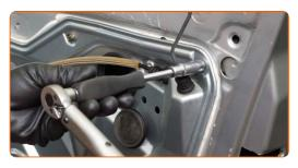
Attach the power window wiring harness.
