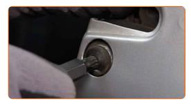
Remove the door panel together with the window regulator linkage.
