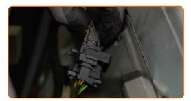
Remove the covers from the window raiser fasteners. Use a plastic trim tool.
