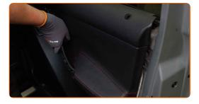
63 Screw in the door card fasteners. Use a Phillips screwdriver.
