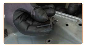
Install the connector holder on the new door panel.
