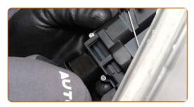
Screw in the door panel fasteners. Use a drive socket #10. Use a ratchet wrench.
