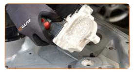
28 Install the power window motor.
