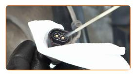
Attach the ABS sensor connector.
