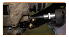
Remove the brake caliper.
