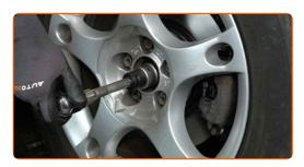
Loosen the wheel bolts. Use wheel impact socket #17. Use a tap wrench.
