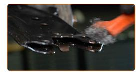
Clean the tie rod end fastener. Use a wire brush. Use WD-40 spray.
