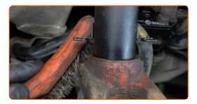
Unscrew the lower fastener connecting the shock strut to the steering knuckle. Use a drive socket #18. Use a combination spanner #18. Use a ratchet wrench.
