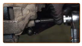
79 Install the caps on the brake caliper guide pin boots.
