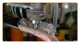
Unscrew the fastening nut connecting the tie rod end to the steering knuckle. Use a drive socket #19. Use a ratchet wrench.
