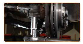
Tighten the lower fasteners of the suspension strut. Use a drive socket #18. Use a torque wrench. Tighten it to 50 Nm torque.+90°
