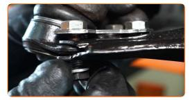
Tighten the fasteners that connect the ball joint to the suspension arm. Use a drive socket #13. Use a ratchet wrench.
