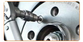
Clean the brake caliper bracket of dirt and dust. Use a wire brush. Use a brake cleaner.
