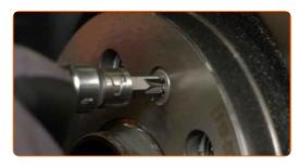
15 Remove the fastening bolt.
