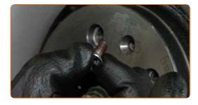
16 Remove the brake disc.
