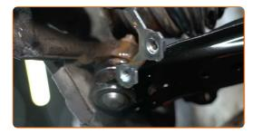
Detach the driveshaft from the steering knuckle.
