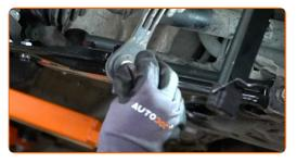
Tighten the fastener connecting the sway bar link to the suspension arm. Use a drive socket #16. Use a torque wrench. Tighten it to 30 Nm torque.
