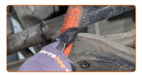
Unscrew the fastener connecting the stabilizer link to the control arm. Use a drive socket #16. Use a ratchet wrench.
