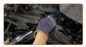
Unscrew the rear fastener of the control arm. Use a combination spanner #18. Use a drive socket #18. Use a ratchet wrench.
