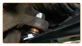
Support the steering knuckle. Use a hydraulic transmission jack.
