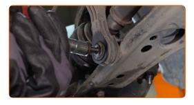
Remove the fastening bolt.
