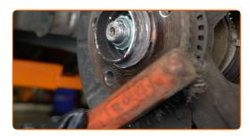
Treat the contacting surface. Use ceramic grease.
