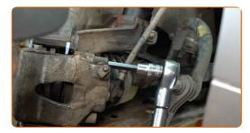
Install the caps on the brake caliper guide pin boots.
