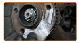
19 Install a new brake disc.
