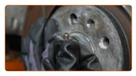
15 Remove the brake disc.
