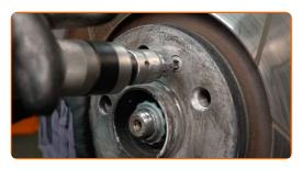
Remove the fastening bolt.
