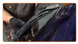
Remove the blade from the wiper arm.
