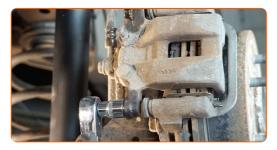
10 Remove the brake caliper.
