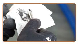
Lubricate guide pins with special brake grease.
