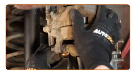
Tighten the brake caliper bracket. Use a drive socket #19. Use a torque wrench. Tighten it to 84 Nm torque.
