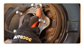
24 Install the brake disc.
