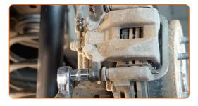
10 Remove the brake caliper.
