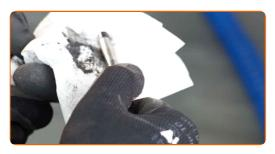
Lubricate guide pins with special brake grease.
