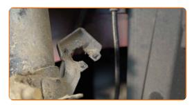
Clean the fasteners connecting the stabiliser link to the shock strut, and those connecting the shock strut to the steering knuckle. Use a wire brush. Use WD-40 spray.
