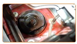
Loosen the upper fastener of the shock strut mount. Use a drive socket #13. Use a ratchet wrench.
