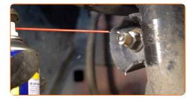
Unscrew the nut and remove the stabilizer rod from the shock strut. Use a drive socket #18.
