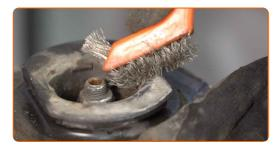
Remove the strut piston rod nut. Use HEX No.H6. Use a drive socket #18. Use a ratchet wrench.
