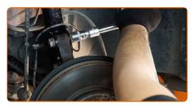
Tighten the fastener connecting the stabilizer link to the shock strut. Use a drive socket #18. Use a torque wrench. Tighten it to 65 Nm torque.
