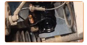
Screw in the fastener that connects the shock strut to the steering knuckle. Use a drive socket #21. Use a combination spanner #21.
