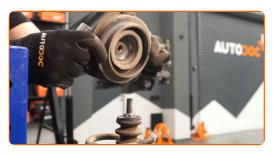
Release the coil spring.
