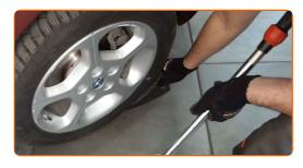
Remove the fender protection cover.
