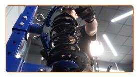
Remove the assembled shock strut.
