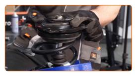
Tighten the shock strut piston rod nut. Use a drive socket #18. Use HEX No.H6. Use a torque wrench. Tighten it to 68 Nm torque.
