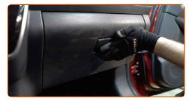
Install and secure the protective cover under the glove box.
