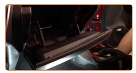
Unscrew the glove box fastening screws. Use a Phillips screwdriver.
