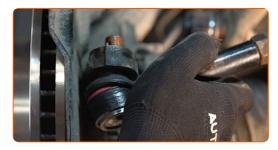
Tighten the fastening nut connecting the tie rod end to the steering knuckle. Use a drive socket #19. Use a torque wrench. Tighten it to 91 nm torque.
