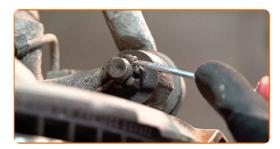
Unscrew the end fastening nut to the steering knuckle. Use a drive socket #19. Use a tap wrench.
