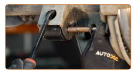
Tighten the fastener connecting the trailing arm to the car body. Screw in the fastener connecting the control arm to the rear subframe. Use a combination spanner #19.
