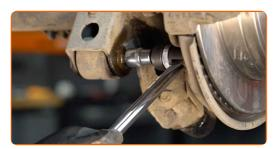
Unscrew the fastener connecting the trailing arm to the car body. Use a combination spanner #19. Use a drive socket #19. Use a tap wrench.
