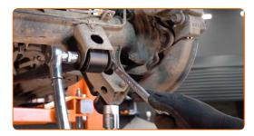
Tighten the fastener connecting the control arm to the car body. Use a combination spanner #19. Use a drive socket #19. Use a torque wrench. Tighten it to 130 Nm torque.
