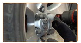
Lower the car and working in a cross order, tighten the wheel bolts. Use a torque wrench. Tighten it to 112 nm torque.
