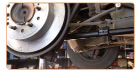
Tighten the arm fastening to the beam. Use a combination spanner #19. Use a drive socket #19. Use a torque wrench. Tighten it to 130 Nm torque.
