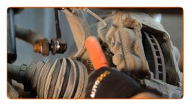
Unscrew the brake caliper fastening. Use a drive socket #17. Use a tap wrench.
