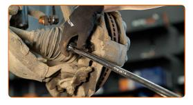
Remove the brake caliper.
