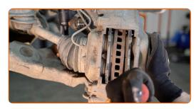
Remove the brake pads.
