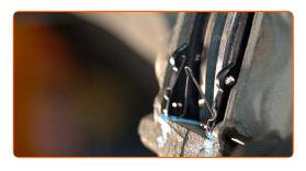
Install the brake pads retaining clips.
