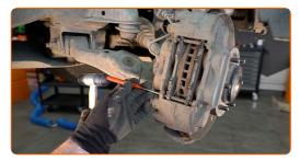
Remove the retaining spring of the brake pads.
