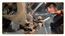
Secure the brake hose fastening bracket. Use a drive socket #12. Use a ratchet wrench.
