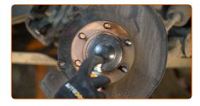
21 Install the brake disc.
