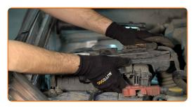
Remove the fender protection cover.
