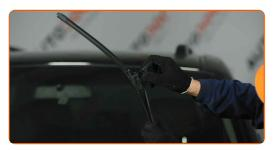
Remove the blade from the wiper arm.
