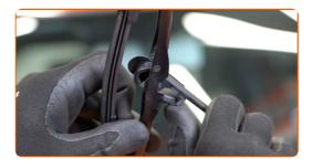
Remove the blade from the wiper arm.
