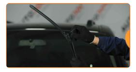
Remove the blade from the wiper arm.
