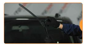
Remove the blade from the wiper arm.
